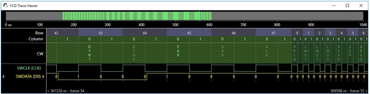
Time is given in **ns** and in frame ID. The data line BitSlots are shown in their LOGICAL form and drawn in their NRZI form. If the VCD file contains other traces, not directly related to the SoundWire traffic, they can also be displayed.
