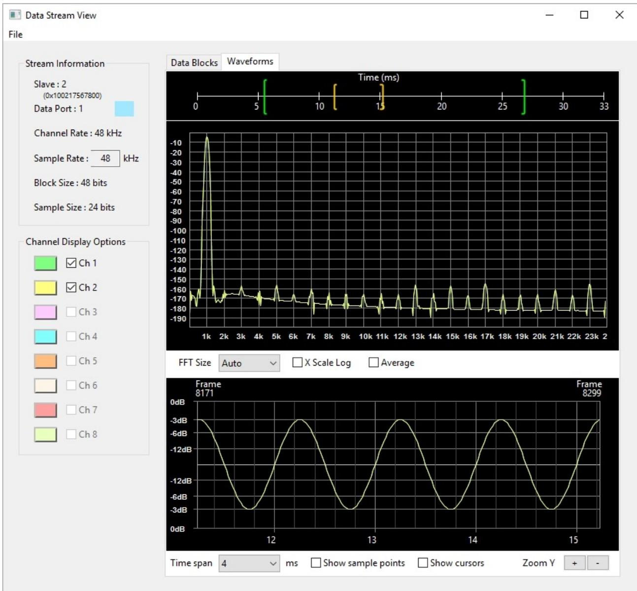
When set to Auto, the FFT size will be computed to be the maximum usable on the data stream.
