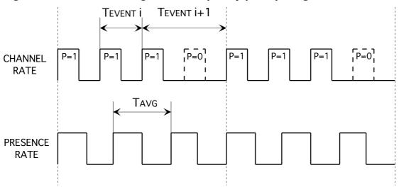
As all the delays are cumulative, the Jitter function **J** is equal to:
